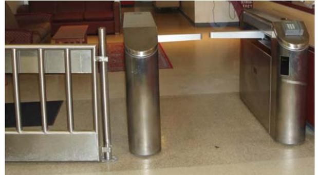
In process, when an unauthorized person enters the unsecured side of the lane, the alarm sensor detects the person. An audible alarm sounds, and the barrier arm is locked into place so that a person cannot force his/her way through the lane. A security officer then directs the student or visitor out of the lane. The officer resets the lane and then guides the person through the proper procedure while the flow of traffic continues with minimal interruption.
